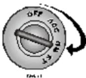
To override the starter kill, turn the ignition on and press the Valet button within 10 seconds. The vehicle should start. If it does not start, you may have
