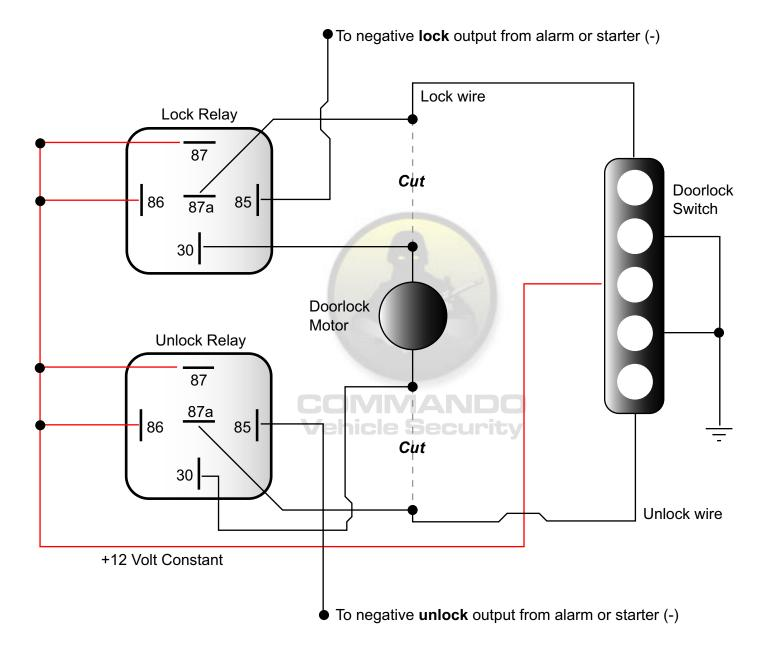
This doorlock system has the factory doorlock switches wired directly to the motors in the doors. All wires at the doorlock switch rest at ground with the exception of the 12 Volt supply wire. When the doorlock switch is activated, one of the circuits is opened and 12 Volts is sent to the motor to lock or unlock the doors.
