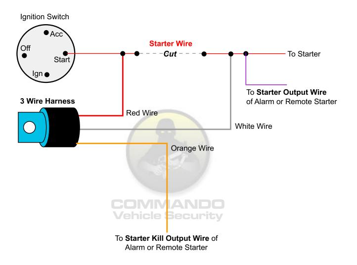
Find the wire in the Ignition Harness that shows +12 Volts **ONLY WHEN CRANKING!**Cut that wire in two and insert the 3 Wire Relay and Socket as shown above.
