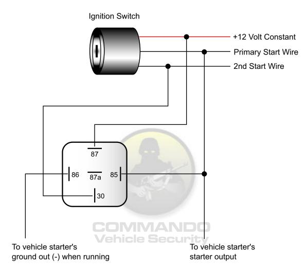
This configuration is used for vehicles equipped with a second starter wire that must be connected for remote start.
